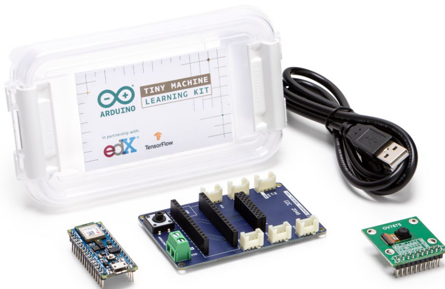
Figure 3. Le kit Arduino Tiny Machine Learning comprend une carte Nano 33 BLE Sense.
