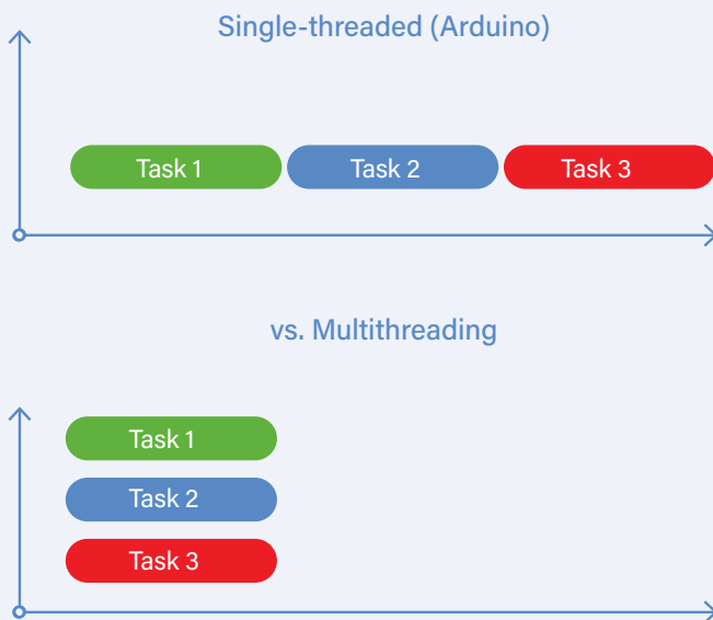
Figure 1. Fil unique ou fils multiples, mono-thread vs. multithreading.
