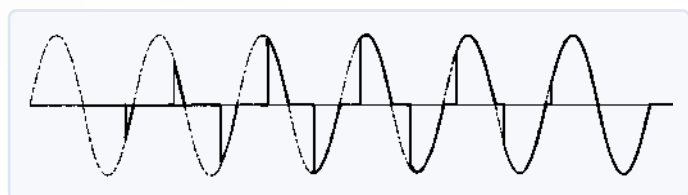
Figure 4. Coupure de phase.
